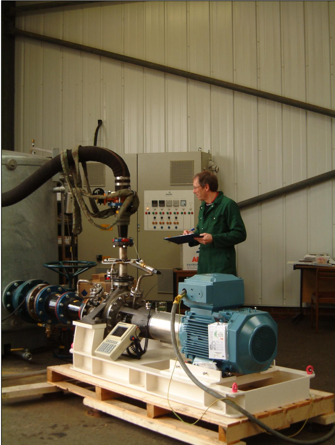
Amarinth testing API 610 OH2 A-Series pump
